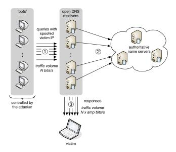
Figure 1: DNS amplification attack
